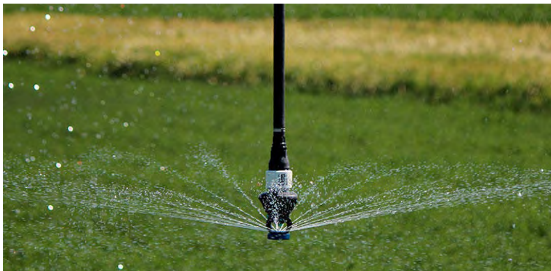
Figure 4.3b – Illustration of LESA low drift sprinkler emitter (senninger.com)
