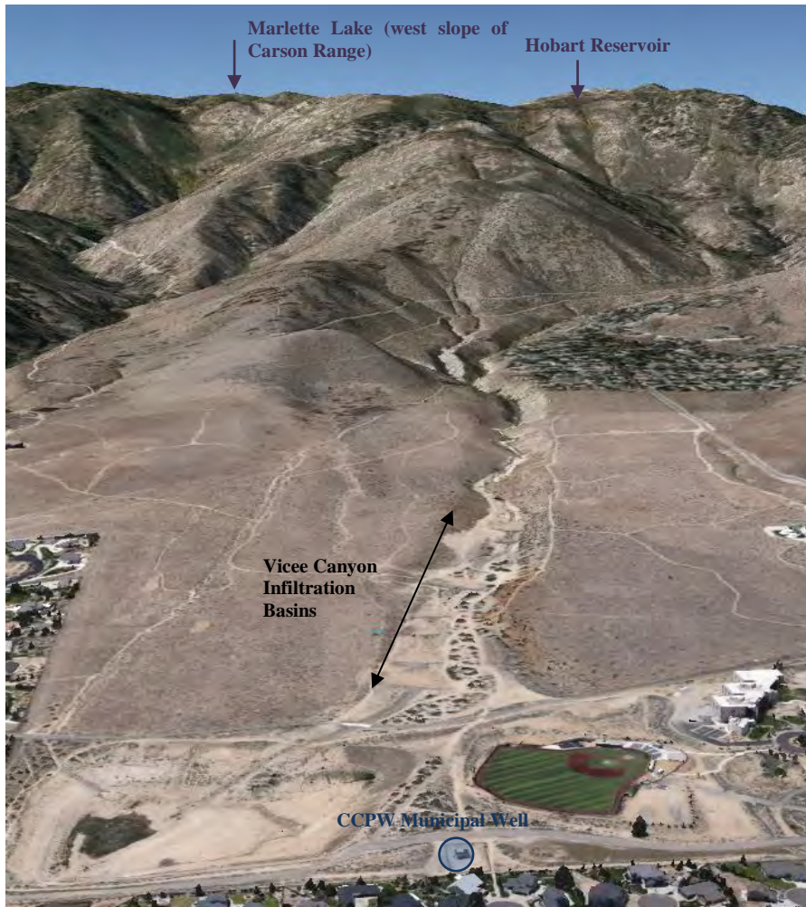
Figure 4.20 - Vicee Canyon and the terraced MAR infiltration basins, oblique Google Earth view facing west toward the Carson Range
