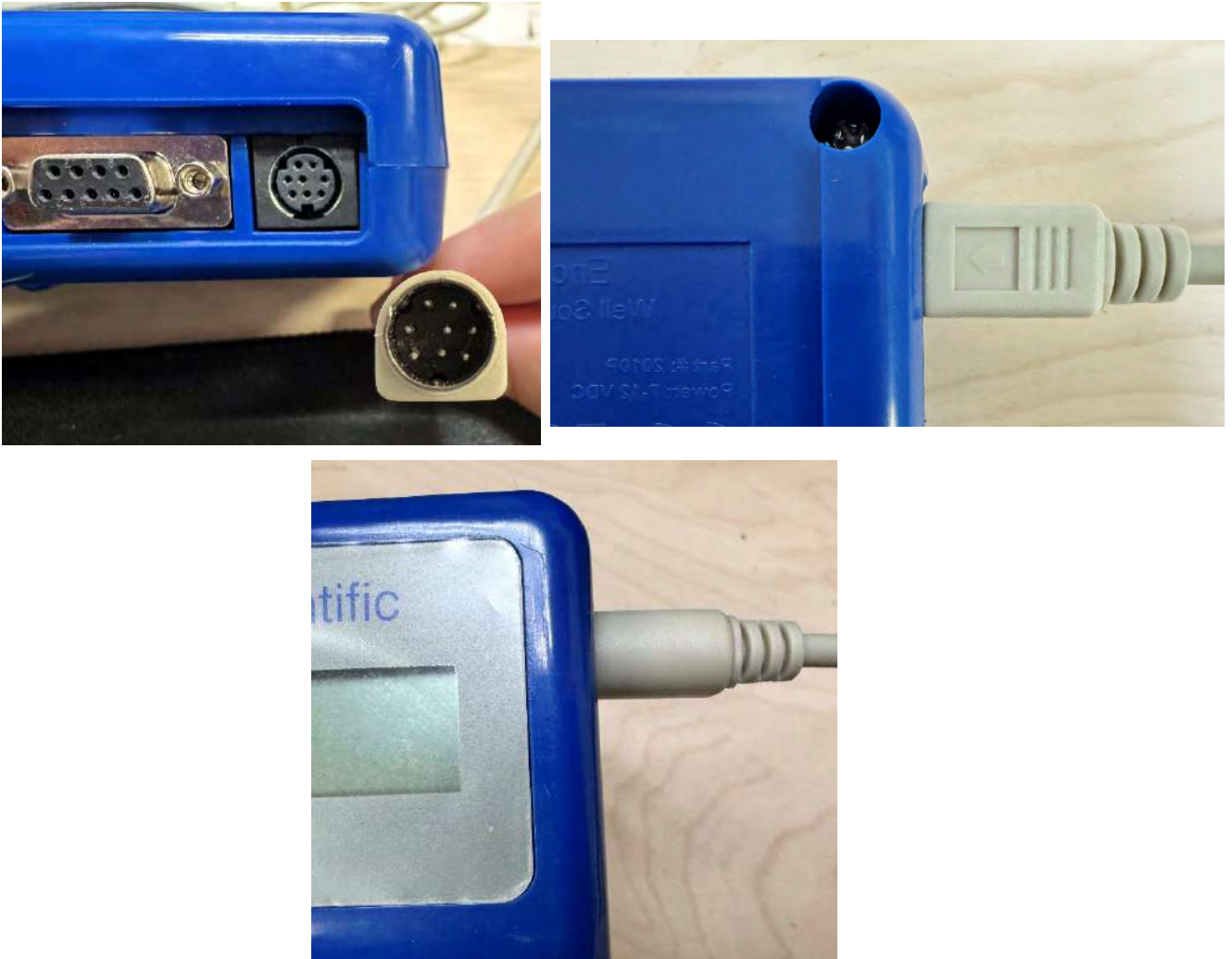
Figure 1. Correct orientation of the cable, with the flat side down. Top is the side with screen and buttons.
