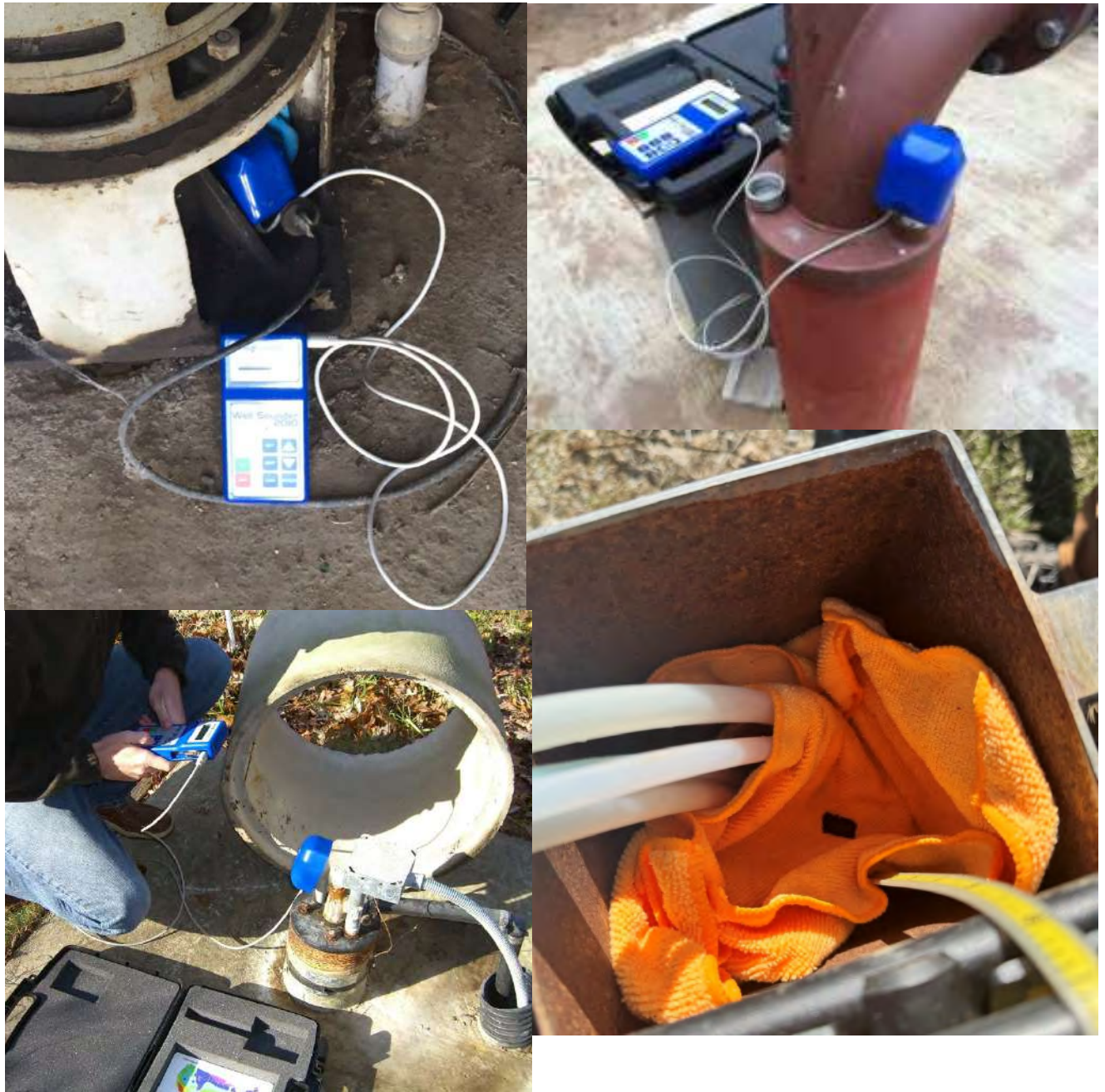
Figure 3. Example sensor setups and example use of cloth to cover a 4 inch well opening, leaving a cut hole for the probe (lower right).
